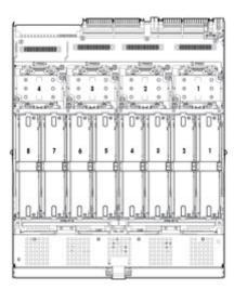
The server can operate in independent channel mode (performance) or combined channel mode (lockstep). Lockstep mode improves the system reliability and availability. If running with RDIMM (built with x4 DRAM devices), the system can survive the complete failure of two DRAM devices (DDDC). Running in independent mode, the server can only survive the complete failure of a single DRAM device (SDDC).
